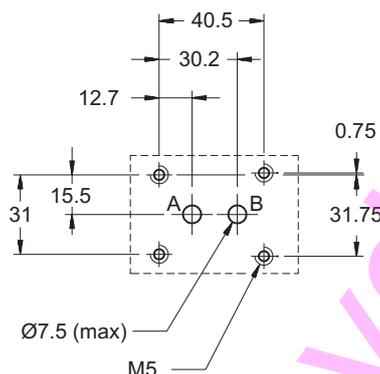
**NOTE:** The RPCED1 mounting interface, with CETOP 03 holes, must not have P and T ports or **must** have the 0113388 subplate (see paragraph 9)
