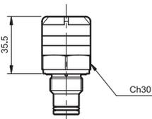
This indicator measures the differential pressure between the filter input and output.
