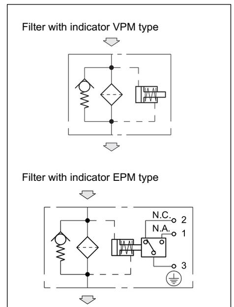
**NOTE 2: The filter size has to be selected so that with the nominal flow rate the pressure drop is lower than 0.8 bar.**
